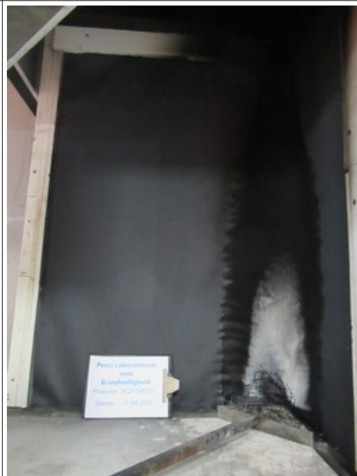
Test specimen 03: EB01 – Black Long wing outer edge after testing
